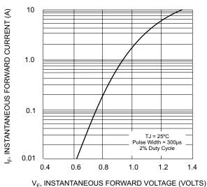
V<sub>F</sub>, INSTANTANEOUS FORWARD VOLTAGE (VOLTS) Fig. 2 Typical Forward Characteristics
