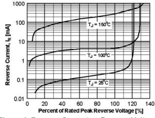
Figure 4. Reverse Current vs Reverse Voltage
