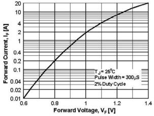
Figure 2. Forward Voltage Characteristics
